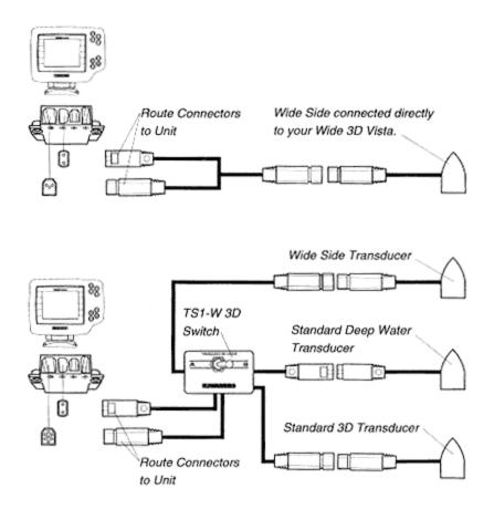
When the Wide Side transducer is connected directly to your unit, or selected using a transducer switch, the unit setup must be changed to correspond with the type of transducer being used. This adjustment is made through the "System Options" menu. Use the MENU button to select the "System Options" menu and press ENTER. Press MENU until the "sonar mode" option is highlighted. Press UP or DOWN until "side" is displayed. Press ENTER when the selection is correct.
